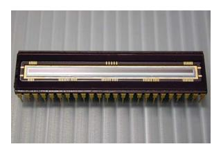
Each horizontal register is connected to a highspeed output amplifier. The output amplifier is a three-stage source follower designed for high conversion gain and extended bandwidth.
